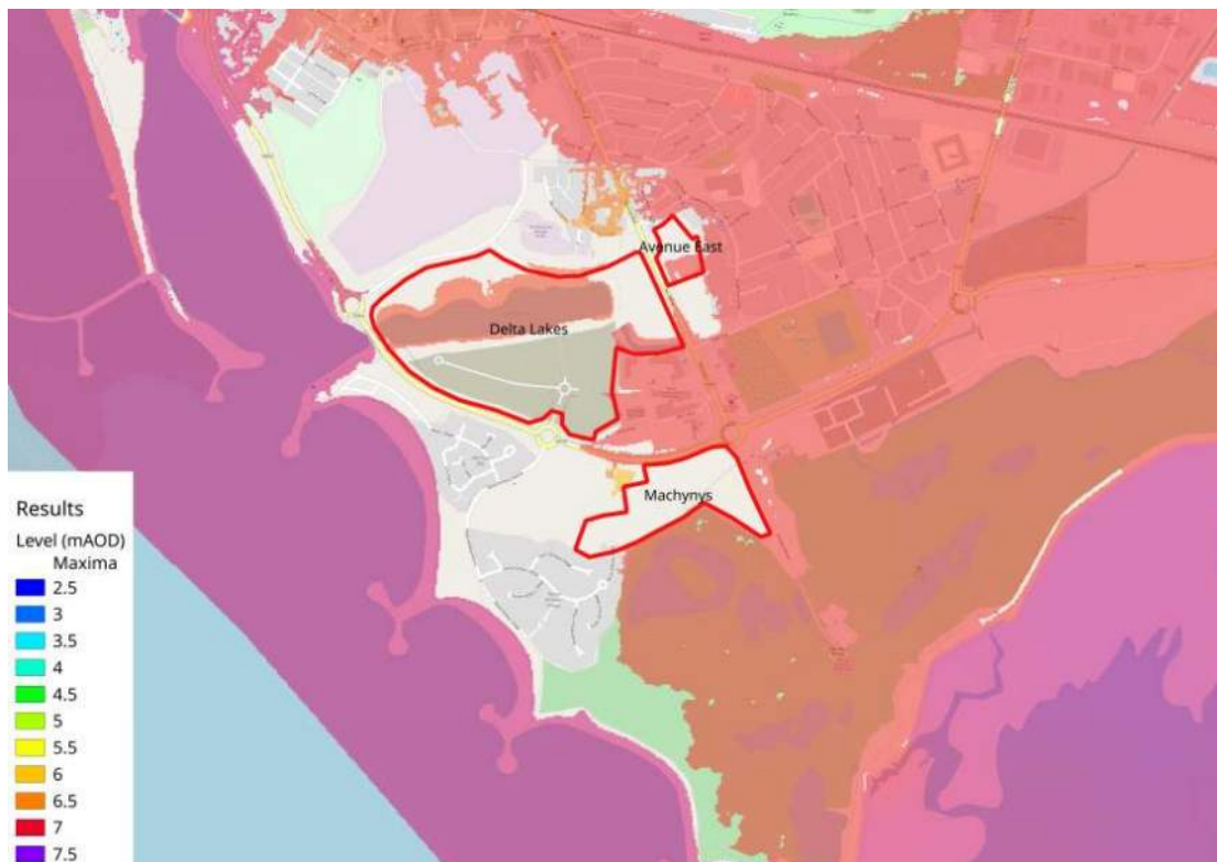
Figure 4.3: Post-development Model Results - Peak Water Level for a 0.1% AEP tidal /surge event in conjunction with a fluvial flow of QMED with 75% Climate Change
