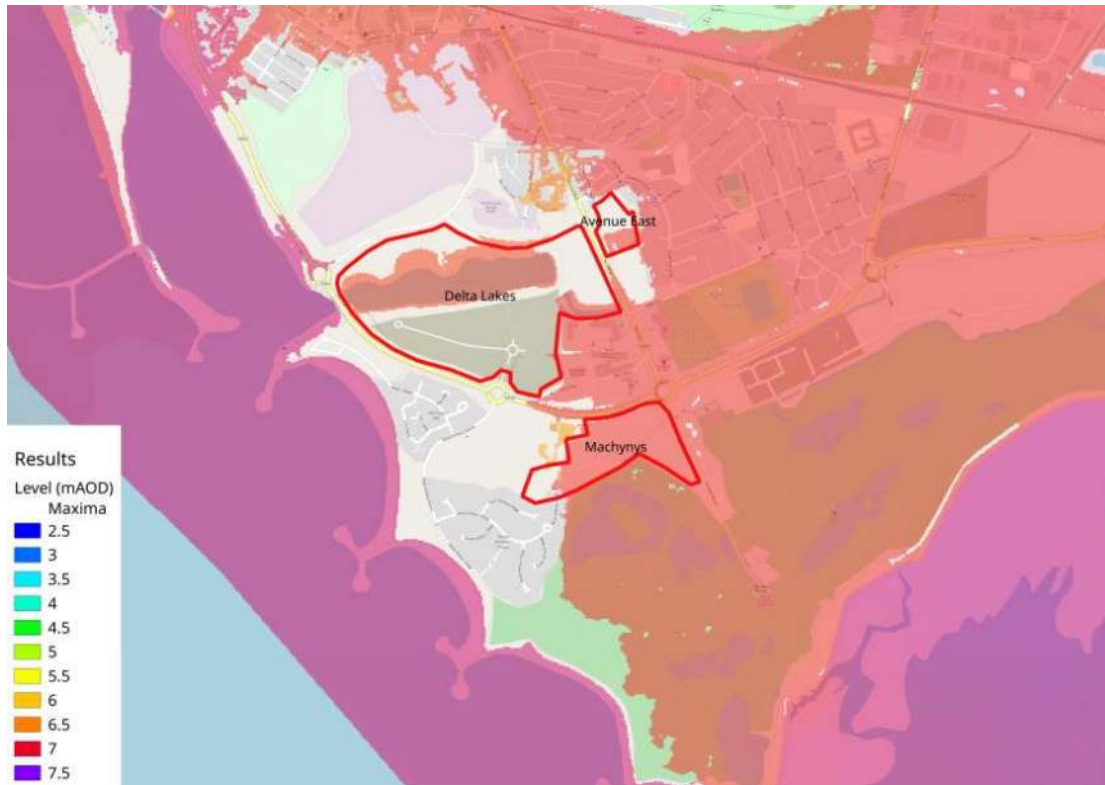
Figure 4.2: Pre-development Model Results - Peak Water Level for a 0.1% AEP tidal /surge event in conjunction with a fluvial flow of QMED with 75% Climate Change
