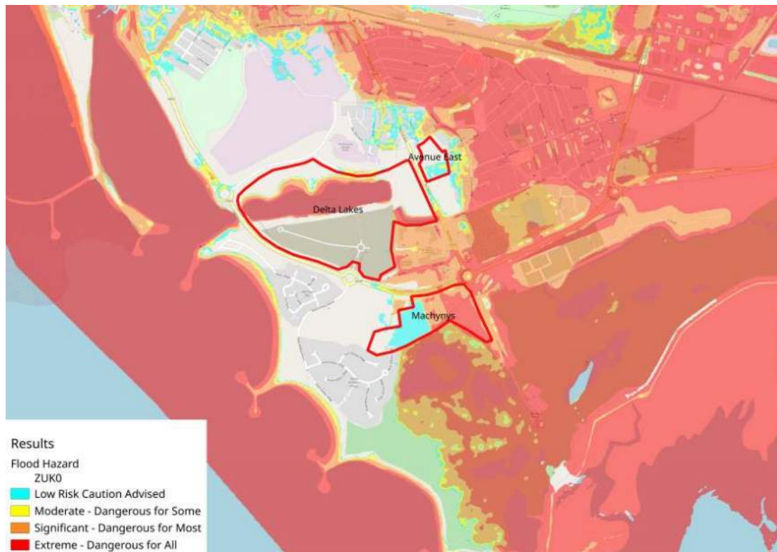
Figure 4.6: Pre-development Model Results - Peak Hazard for a 0.1% AEP tidal /surge event in conjunction with a fluvial flow of QMED with 75% Climate Change
